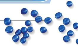
**Polytrope<sup>®</sup> STR** Series 1000 and 2000 are based on enhanced polyolefin compositions that have been specifically designed to provide high melt strength for sheet extrusion and thermoforming applications. *Polytrope<sup>®</sup> STR* Series 1000 and 2000 can be categorized within the thermoplastic polyolefin (TPO) family of polymers. As such, they can be painted using the same materials and procedures commonly associated with painting TPO.
